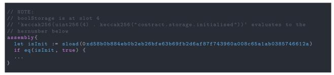
While this is possible to do using inline assembly, it is clearer and less error prone to simply store the initialised flag as a standalone state variable (and thus stored at a small-integer storage location).
